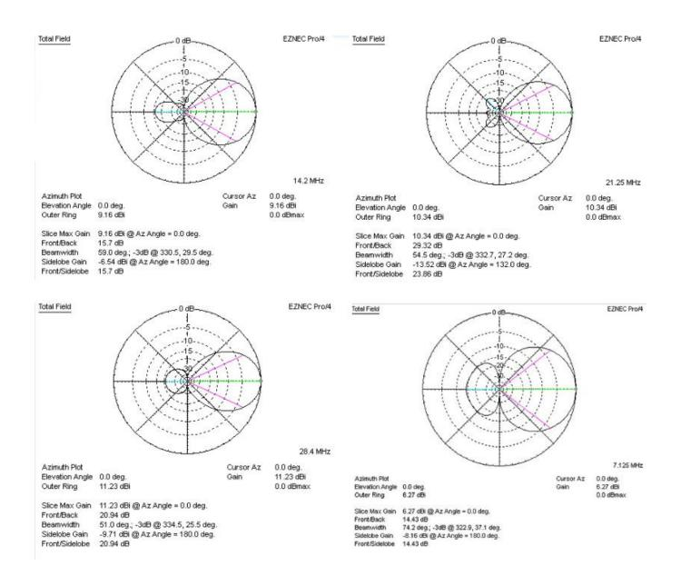
TYPE B : Two Element 40M Yagi - 18ft Boom
